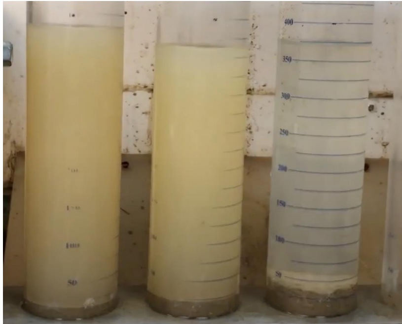
Image: Left to right; control, polymer flocculant only, coagulant and polymer.
