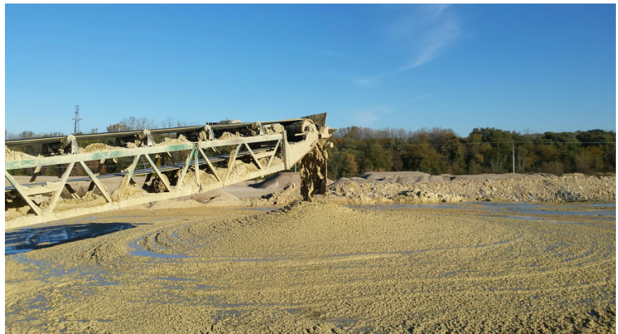
The clarification system has dramatically increased the percentage of solids in the discharge. The thickened mud, at an estimated 68 percent solids, is transferred to a containment area where it dries in less than a week.
