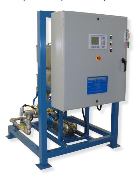
After fifteen years of service the dry polymer batching system for our sludge dewatering presses was badly corroded and repair parts were becoming increasingly tough to find. We didn't need a whole new system as our batch tanks and mixers were still fine. The old machine simply needed a new heart and brain.
